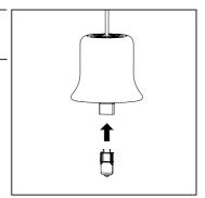
Screw the glass onto the G9 lamp holder.
