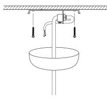
Mount the metal bracket securely in the ceiling with screws and appropriate plugs. Fix the cable in the correct length in the plastic cable lock.
