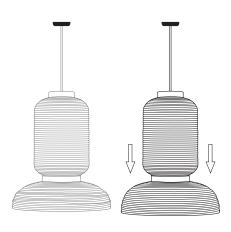
Once the pendant is in place, carefully stretch and adjust the bottom of the shade to make sure paper is fully folded out.
