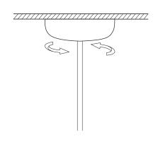
Put the canopy over the metal bracket and twist to lock into place.
