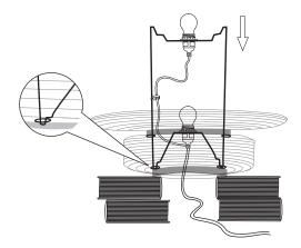
Place the paper shade up-side-down on a raised surface allowing for a gap to pass the cable through. (We recomemend two large books). Then place the top of the frame through the bottom of the shade and into the metal hoops connected to the top of the pendant.
