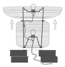
Carefully pull the shade up over the rest of the frame and hook it into the secondary set of hoops.
