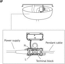
Use the terminal block inside the junction box to assemble the wires from the pendant with the wires from the power supply. Close the junction box and place it inside the canopy.
